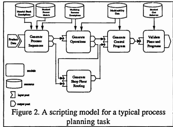
Figure 2. A scripting model for a typical process planning task
