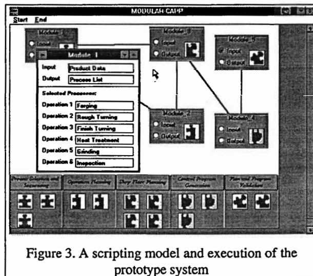
Figure 3. A scripting model and execution of the prototype system
