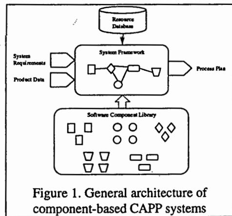
Figure 1. General architecture of component-based CAPP systems
